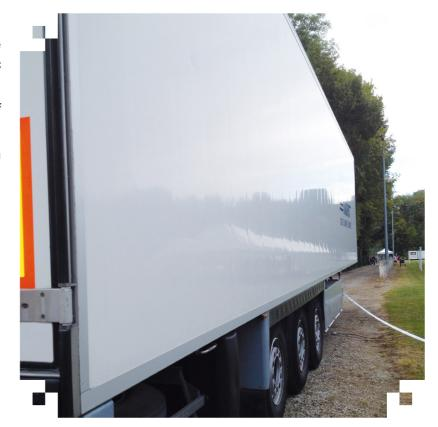
An example of UP Resin's application: composites' panel for transportation
