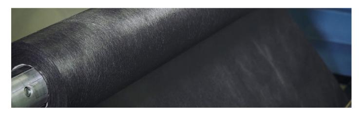
Detail of recycled carbon fiber veil for surface improvement (20 gr/m
