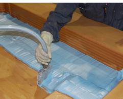
Depositing of tooling paste onto a plug to make a mold.
