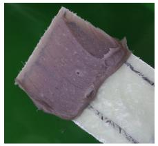
This photo shows the application of Bonding Paste
