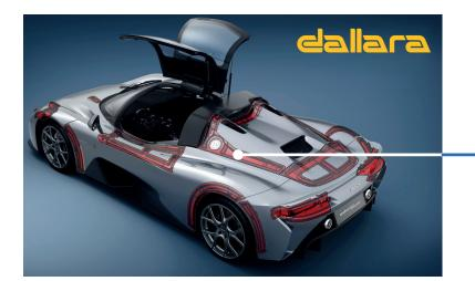
**Compounds for Automotive SMC:** Polynt-SMCarbon<sup>®</sup> used for 9 inner structural parts. (Photo of Dallara Stradale, the new road car of Dallara. Photo by Dallara)
