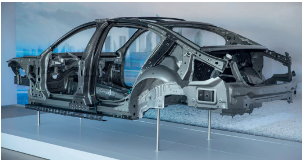
Example of BMW recycled carbon fiber.
