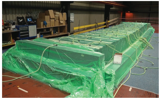
The bridge deck is manufactured as a complete element using a vacuum infusion process
