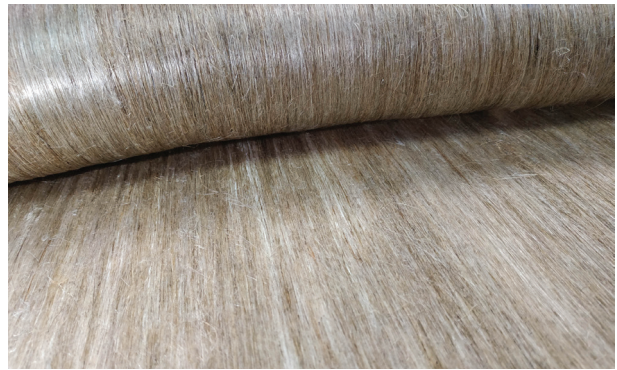
Flax fibres could become a building material of the future. Flax mats combined with bio-resin can be made into a light and highly stable material with properties comparable to aluminium or steel.
