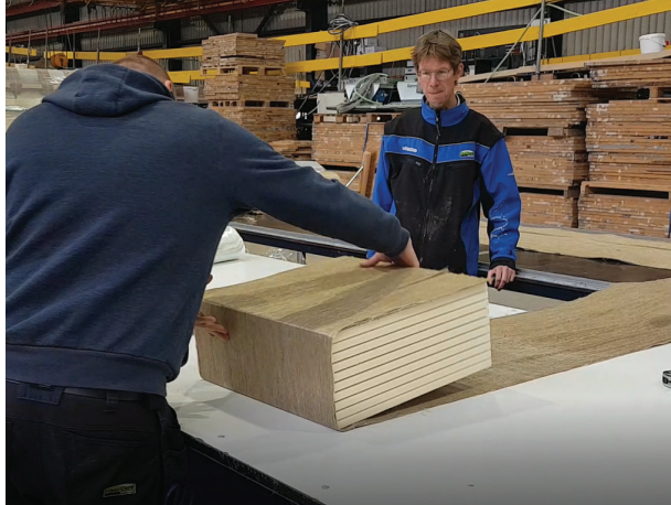
Production process: fibre mats made from flax are wrapped around lightweight foam cores.
