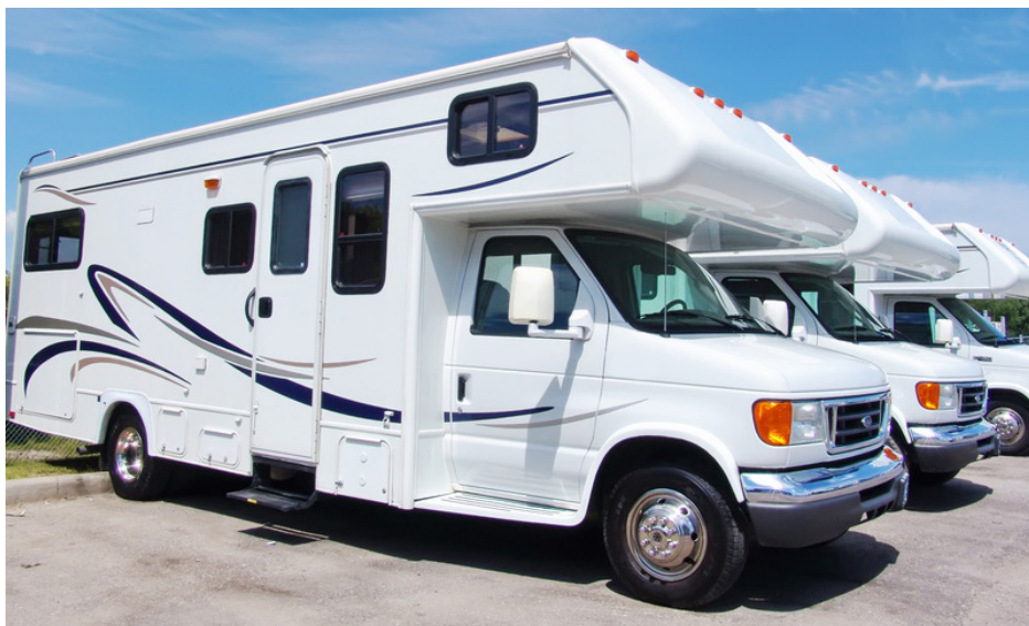
SWIFT motor caravan: the front and rear bumpers and roof of caravans and campervans are made of Optimold Tooling (and tooling gel coat).
