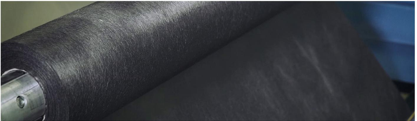
Detail of recycled carbon fiber veil for surface improvement (20 gr/m)
