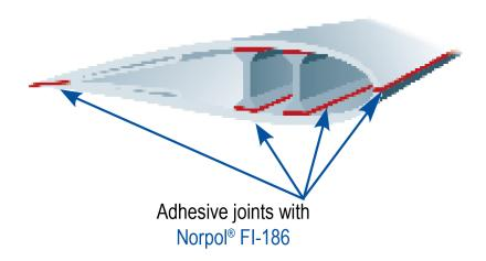
The Norpol FI-186 bonding paste recommended for use on rotor blades is approved by DNV GL. Some of the tests performed for wind blades bonding paste include:
